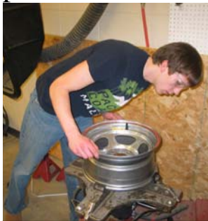
Nick clamping the hub in place
